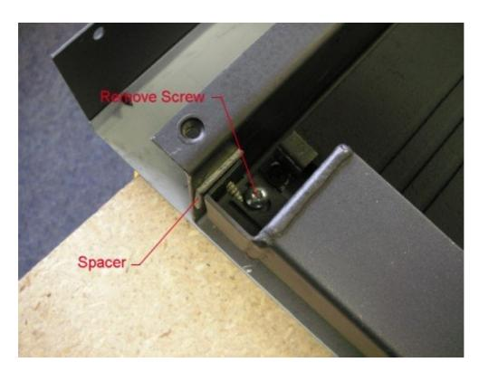
Twist the LH end of the burner by pivoting on RH screw until clear of the body, then pull burner out.. retaining lug is slotted.
