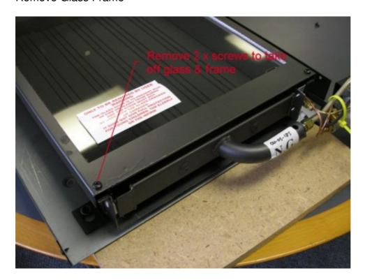
Remove LH mounting screws – leave RH screw as you cannot get to it.
