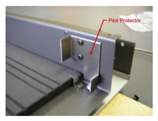
Fit Pilot Protector – only used with NG burner – before reassembling.
